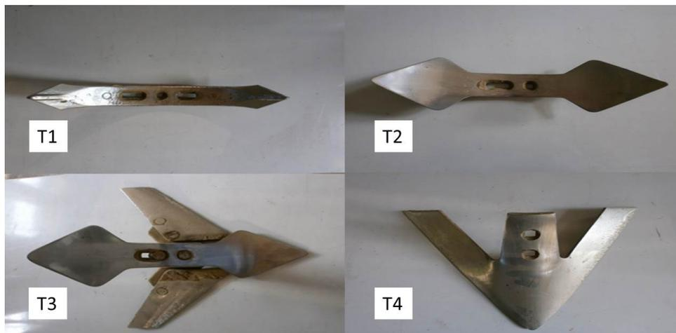
Figure 1: Standard single tines used in the experiment (© A. Al-Neama)
