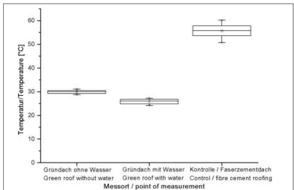
Fig. 2: Distribution of temperature measures at the bottom side of the green roof compared to control without green roof
