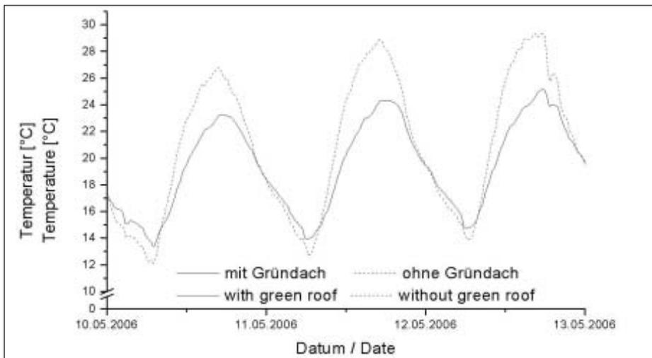
Fig. 1: Profile of daily temperature measures inside the stable of the green roof and roof without plants in May 2006
