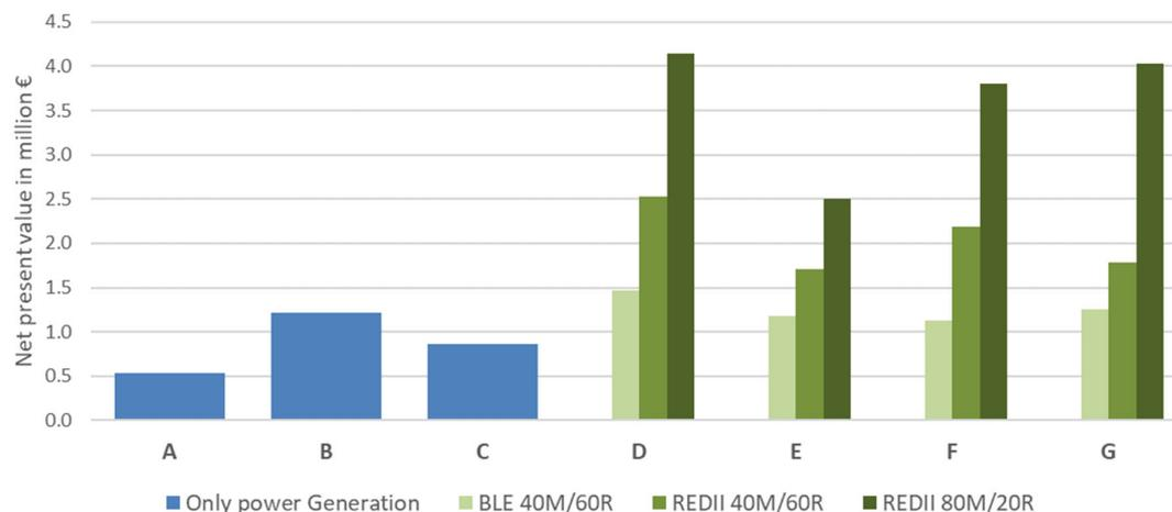
Figure 8: Comparison of the overall profitability of the seven connection scenarios for a 500 kW<sub>el,inst</sub> BGA – scenarios A to C with electricity generation only, D to F with proportional electricity and fuel production and G with complete fuel production
