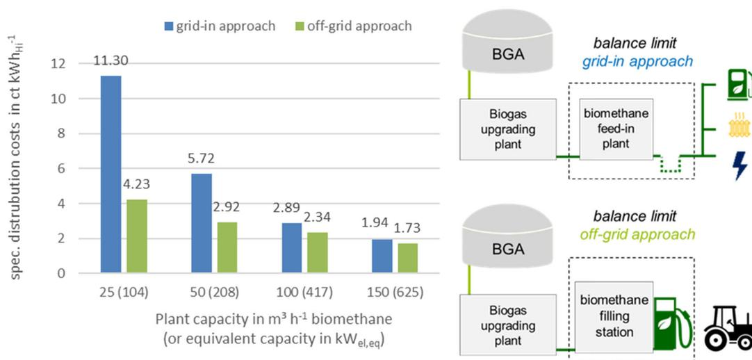
Figure 2: Specific cost comparison of the distribution approaches grid feed-in and off-grid approach for biomethane (grid feed-in costs from eMikroBGAA (BEIL and DANIEL-GROMKE 2019), off-grid costs own calculation)
