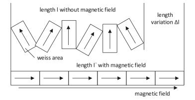
Figure 6: Joule effect: Length variation of a ferromagnetic part caused by a magnetic field (HERING 2012)
