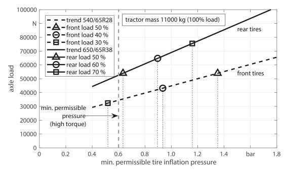
Figure 2: Axle loads (addition of 2 tires) and appropriate minimal tire inflation pressure for various axle load distributions for a middle range standard tractor equipped with Michelin Multibib tires
