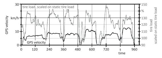
Figure 10: Load on the rear right tire of an Arion 550 equipped with a semi-mounted cultivator and 900 kg front ballast
