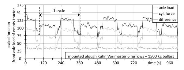
Figure 9: Difference of axle load and calculated cylinder force, measured with an Axion 840 equipped with a 6 furrow plough and 1500 kg front ballast
