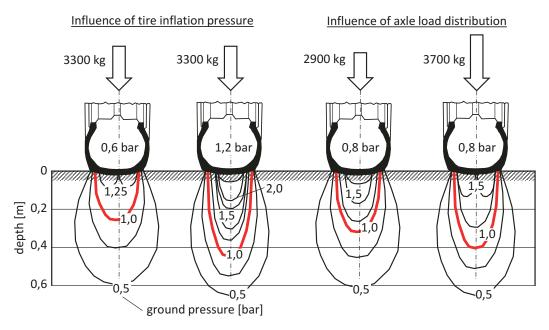
Figure 1: Pressure bulbs beneath a tire Michelin Multibib 650/65R38 on dry secondary podsol (CH7) for various tire loads (left) and various contact area (right), calculated with the soil-compaction-model Terranimo (STETTLER et al. 2014)
