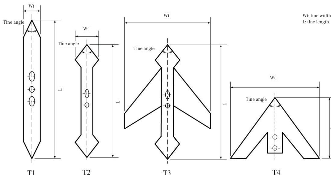
Fig. 1: Tine shape and dimension
