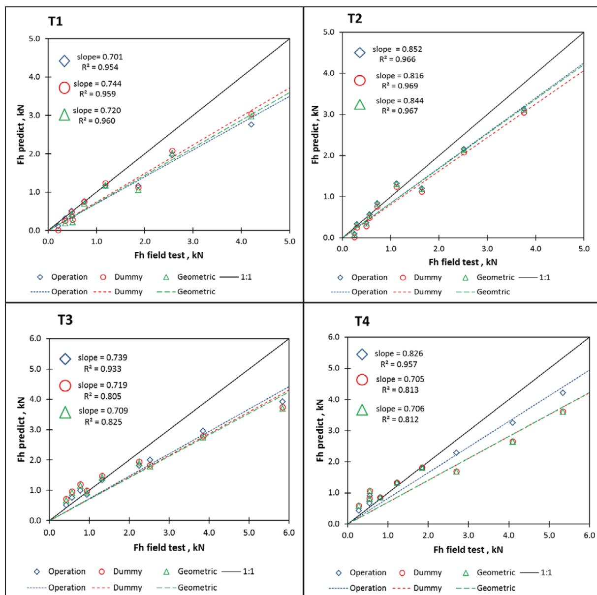
Fig. 2: Comparison of the observed and predicted Fh for all tines
