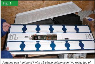
Antenna pad (,antenna') with 12 single antennas in two rows, top of the antenna is removed (Photo: S. Gebhardt-Henrich)
