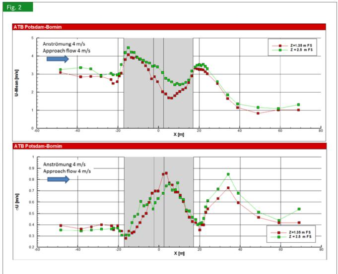
Measured profiles of the mean wind component U in x-direction (above) and the standard deviation  $\sigma$ U (below). Grey area indicates area of the barn including feeding alley in the center.
