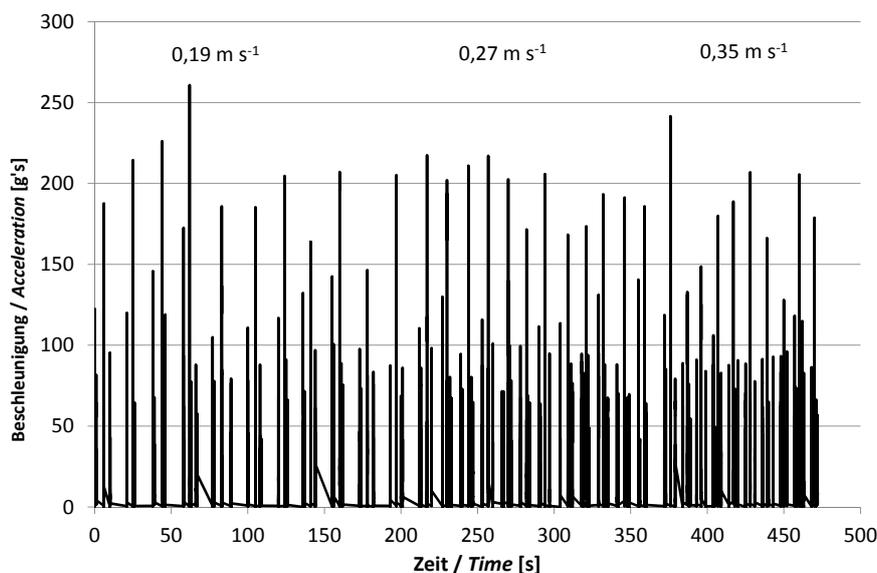
Measurement of impact acceleration with Mikras implanted in a potato Karlena (170 g) running through the processing line simulator (3 conveyor speeds, each ten runs)
