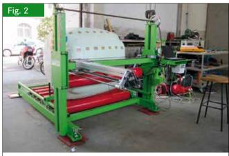
Penetrometer unit of the test bench in front view (Photo: Büscher)
