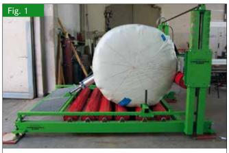
Test bench for measuring the bale density in side view. The bale is rotated by the electric driven roles below. (Photo: Büscher)
