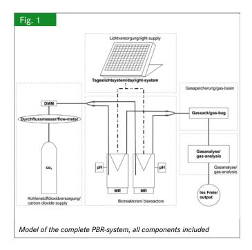
the first test the pH value and the temperature is measured all 60 minutes. At the same time during the filling of the gasbag with  $CO_2$  measurements for  $CO_2$  and  $O_2$  concentration were collected every second, later on all 30 seconds. In addition the gas analysis recorded surrounding temperature and pressure.
