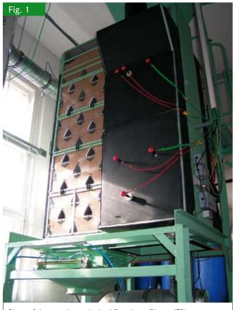
Photo of the experimental mixed-flow dryer (Photo: ATB)
