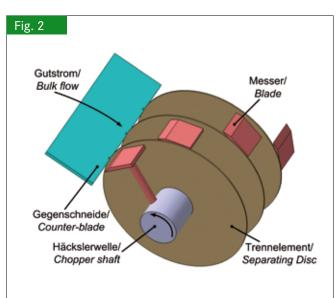
Cutting device with integrated separating discs
