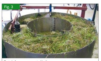
Test rig for measurement of bulk crop
