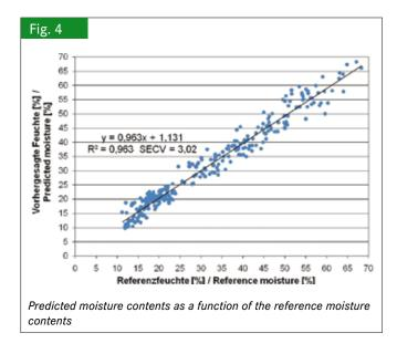
was 3.02 %. The coefficient of determination  $(R^2)$  is 0.96. The undervaluation (bias) in the samples was very low. The evaluation of the bale measurement results, however, yielded higher discrepancies.
