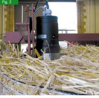
Measuring head installation for radial measurements on bales
