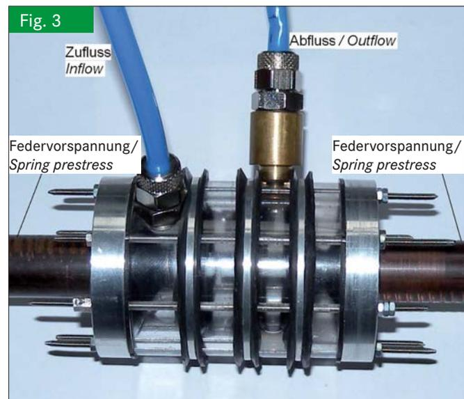
Pressure-driven flow valve (fv). Water flow through the fv is disabled but possible within a predefined water pressure range adjusted with springs.
