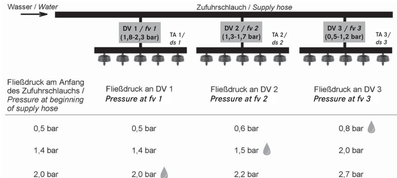
Sketch of the on-farm irrigation experiment (LVWO Weinsberg). Water is fed to the supply hose on plateau position. The dripline sectors (ds) 1 to 3 are irrigated independently by switching the pressure-driven flow valves (fv) 1 to 3 with different water pressures in the supply hose (actual irrigation is indicated with a water drop)
