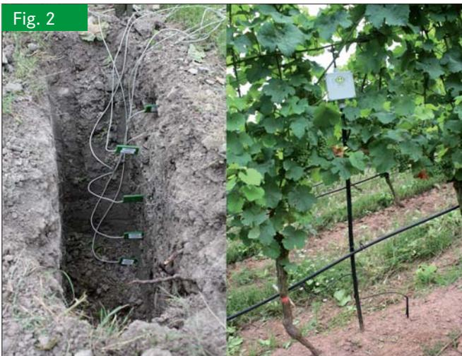
Soil moisture sensors (left) and wireless node for data transfer of soil moisture data (right)
