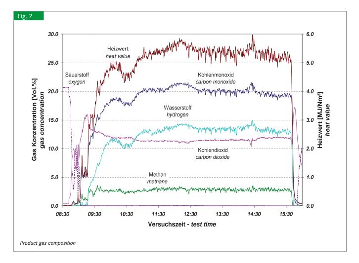
The usage of the cleaned gas for gas turbines or fuel cells is not recommended because of the rest particle content. Additional gas cleaning would be necessary here.
