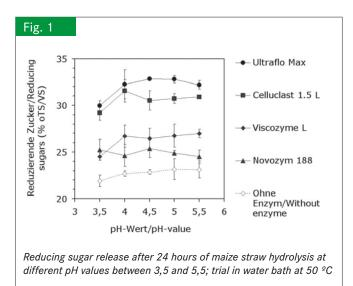
cy of commercial enzyme preparations in degrading maize straw cellulose and hemi-cellulose. Two series of experiments thereby investigated the influence of temperature and pH on enzymatic hydrolysis. As indicator of enzyme efficacy, release of soluble sugars during enzymatic hydrolysis in water medium was recorded via photometric analysis.
