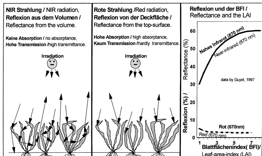
Fig. 4: Reflectance from the volume or from the top-surface
