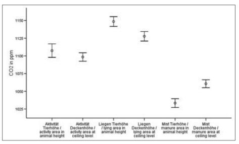
Fig. 1: Carbon dioxide profile versus different measuring sites
