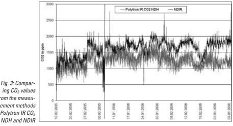
ing CO<sub>2</sub> values from the measurement methods Polytron IR CO<sub>2</sub> NDH and NDIR
