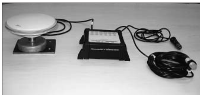
Fig. 1: GPS-data acquisition equipment with additional sensors
