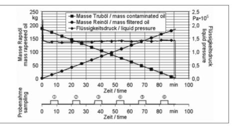
Fig. 1: Alteration of mass and liquid pressure as well as sampling during the filtration of rape oil with a cotton-candle filter
