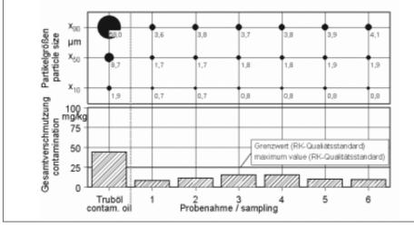
Fig. 2: Particle size and contamination in non-cleaned rape oil and that put through a cotton-candle filter.
