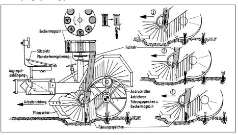
Fig. 3: Planter with revolver-head magazine (plant conveyance directly into the furrow).
