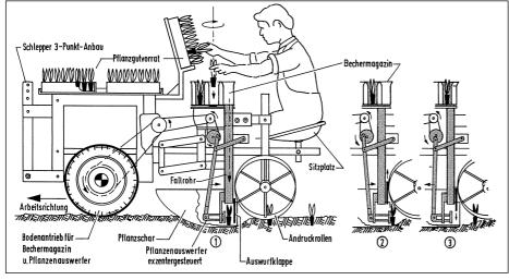
Fig. 2: Planter with revolver-head magazine (plant conveyance in closed coulter)
