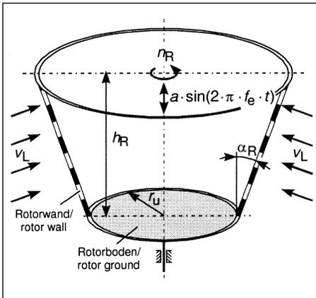
Fig. 1: Structure of rotary cleaning system
