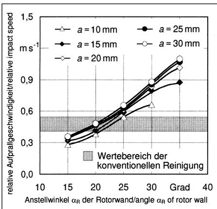
Fig. 3: Relative impact speed of rotary cleaning system
